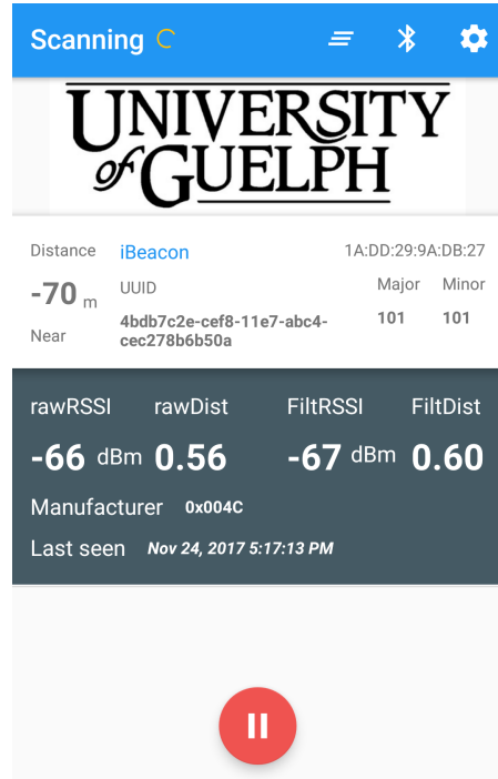
Figure 7: Android Application: Beacon Scanner.
